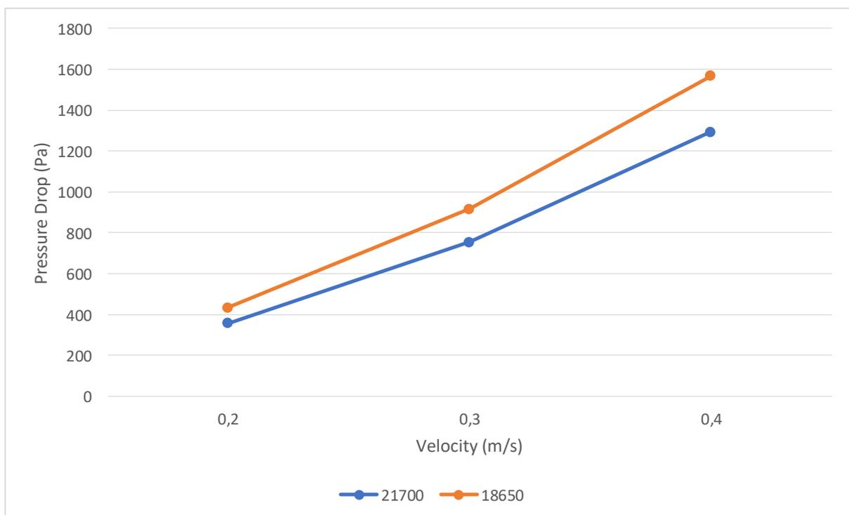
Fig. 9 Variation of pressure drop of coolant
