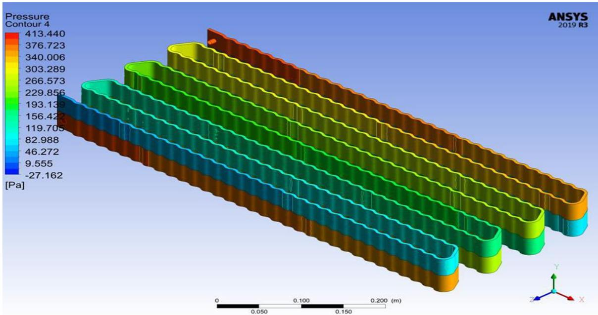
Fig. 3 Effect of 0.25% TiO<sub>2</sub> nanofluid concentration on pressure distribution 0.25% by volume (0.2m/s)
