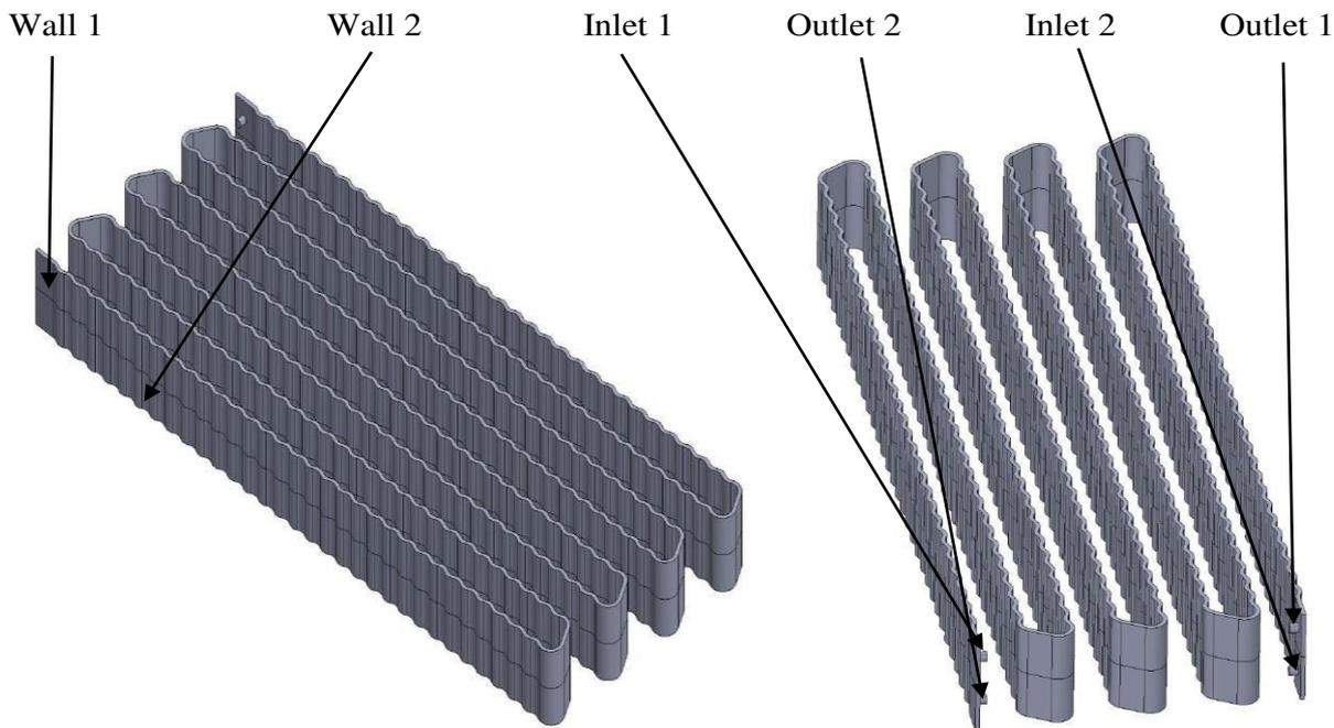
Fig. 1 Battery Cooling Module Of 18650/21700 Battery Cell
